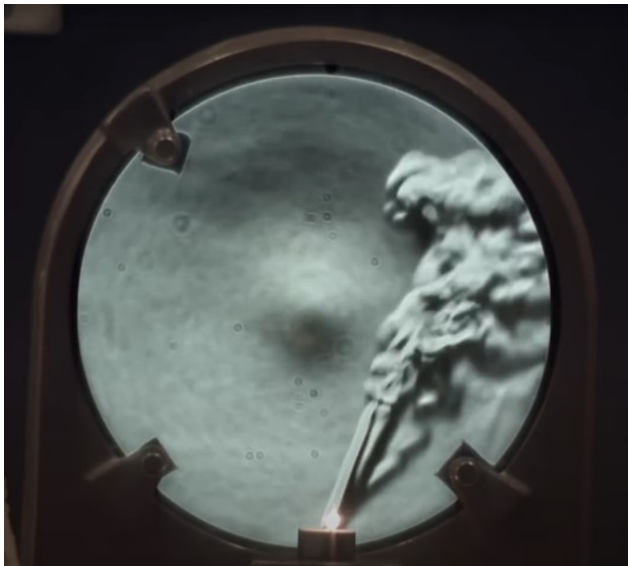
Figure 210: Example of Schlieren Without Color Filters Using a Single Mirror Setup [116]
